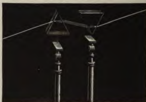
FIG. 40.—Recomposition of white light by means of a second prism.
